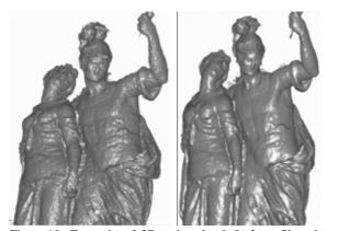
Figure 10: Example of 3D point cloud. Left: unfiltered point data. Right: filtered data using the robust Fast Minimum Covariance Determinant (FMCD) method
