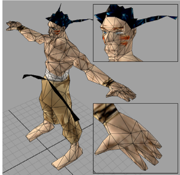
Figure 8: The “Fighter” model reduced to 15% (1044 triangles), using importance weighting
