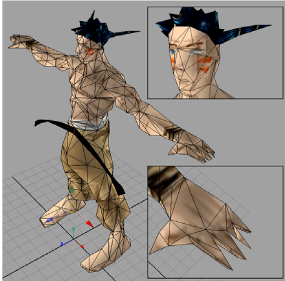
Figure 7: The “Fighter” model reduced to 15% (1044 triangles) with no weighting.
