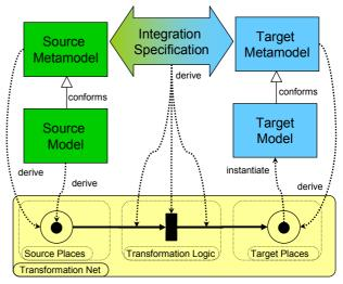
Figure 1. Overall transformation procedure.
