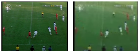
Figure 1.7: Original and encoded frame with reduced bit rate.
