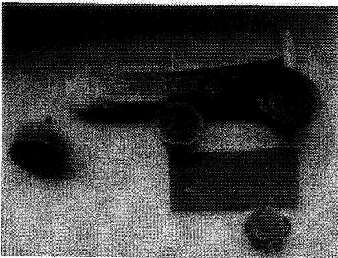
FIG. 3. Replica material to determine the dimension of a corrosion spot.
