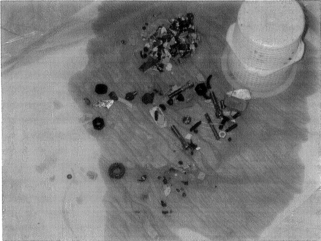
FIG. 8. Collected pieces in the coarse filter.
