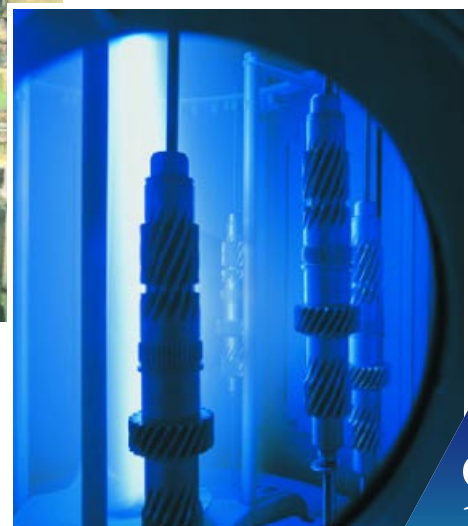
Fig. 19: Highly-demanding HSS tools are often PVD or CVD coated to improve productivity in manufacturing; by courtesy of W. Kalss, Oerlikon, Liechtenstein.
