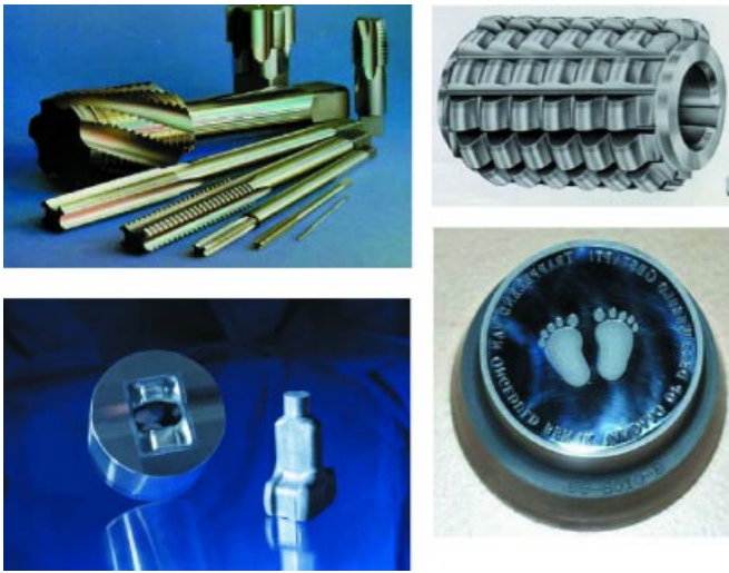
Fig.8: HSS is used for hobs, taps, chasing tools, milling cutters, twist drills but also for cold forming tools (shaping punches, coining and deep drawing dies); by courtesy of Böhler-Edelstahl, Austria.
