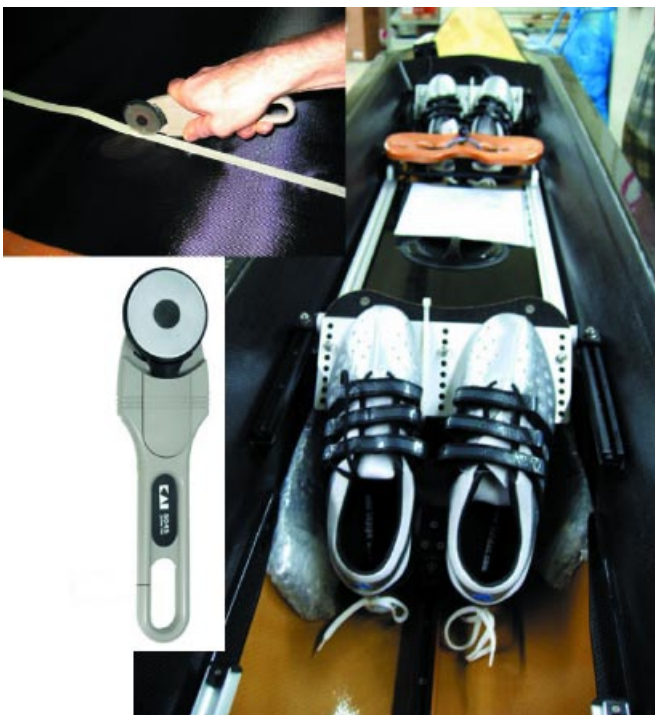
Fig.10: Rotary blade cutters with tungsten steel blades are used for cutting of contoured pieces from multilayer glass and fiber fabrics; pre-fabricated part (rowing boat) made of fiber-reinforced-plastic composite materials; by courtesy of Robuso Solingen and Bootswerft Empacher GmbH; Germany.
