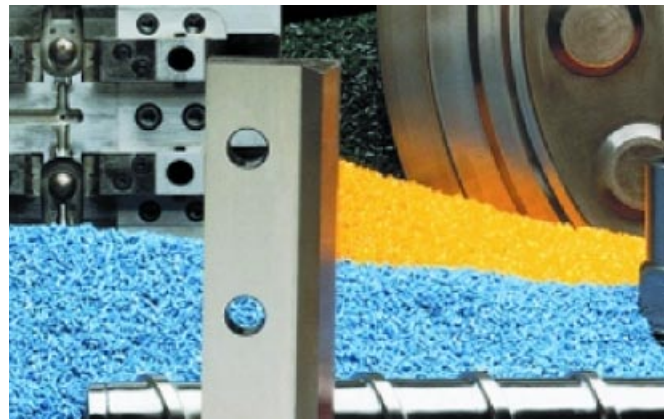
Fig. 17: Tool steel for the plastics industry; screw tip and feed screw for injection molding; the demands on the parts have risen due to the increased use of glass fillers; tools are increasingly made by powder metallurgy technology; CPM®; by courtesy of Crucible Materials Corp.
