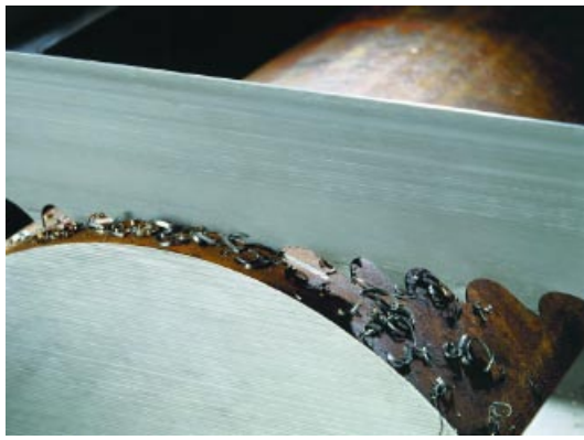
Fig.11: Heavy-duty machining tools are not only used for the machining of steel but also of non-ferrous metals such as nickel-base and titanium alloys; the teeth of the saw blades are made of HSS (M42 bimetal blade); by courtesy of K. Rotbkehl, Wikus, Germany.
