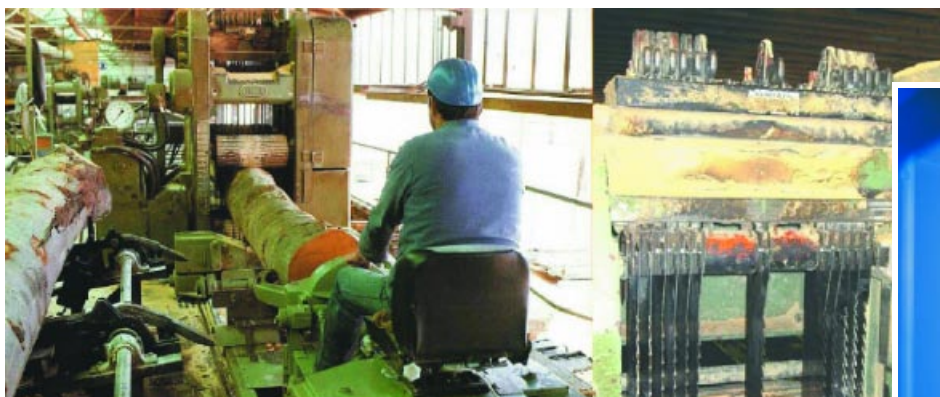
Fig. 18: Gang saw for producing wood boards out of a tree trunk; the saws are made of tool steel which is "stellite" (i.e.: the teeth exhibit an overlay of corrosion resistant tungsten-containing stellite); by courtesy of A. Gaertner, BÖHLER MILLER Messer & Sägen GmbH, Austria
