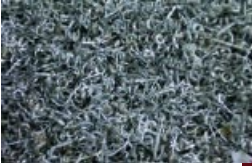
Fig.2: Tungsten is added to the steel melt either as tungsten scrap filled in steel drums, or, alternatively, as ferrotungsten (below); by courtesy of Cronimet, Germany and H. Schulze, Mexico.
