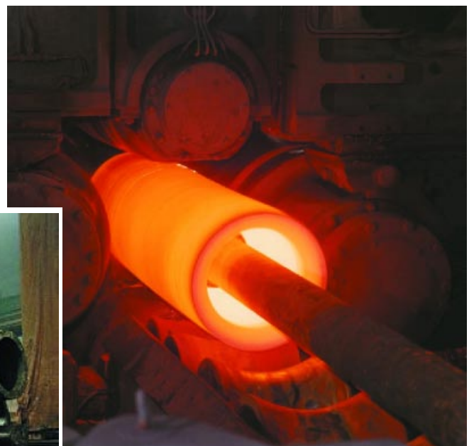
Fig.21: Thick walled seamless pipes of T/P92 materials (X10CrWMoVNb9-2 [max.2% of W]) are produced in a piercing mill according to the Mannesmann process.
