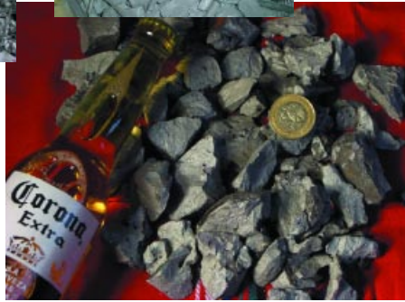
Fig.2: Tungsten is added to the steel melt either as tungsten scrap filled in steel drums, or, alternatively, as ferrotungsten (below); by courtesy of Cronimet, Germany and H. Schulze, Mexico.
