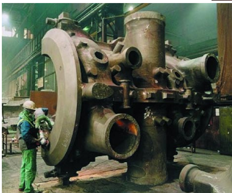
Fig.22: Intermediate pressure inner casing (half), as part of a steam turbine. Weight of the casing is 60 tons. It is made of a martensitic CrMoV-alloyed steel grade containing approx. 1% tungsten (G-X12CrMoWVNbN10-1-1); by courtesy of R. Hanus, voestalpine Giesserei Linz GmbH.
