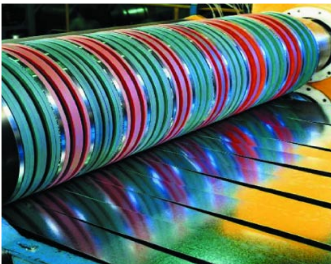
Fig.9: HSS knives are used in large numbers for slitting or transverse cutting of steel tapes, such as tin plate or galvanized sheet; by courtesy of M. Gstettner, Böhler Miller Messer und Sägen GmbH, Austria.
