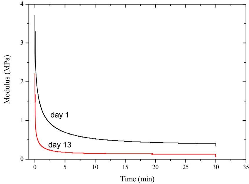
The degeneration of the mechanical behaviour can be explained by the reduction of the PGs between the measurements of the cfc samples. The half-life period was exceeded several times, leading to the significant reduction of the PG concentration. Additionally, the chondrocytes were also no longer vital at the time of the second measurement leading to further degradation of the material.
