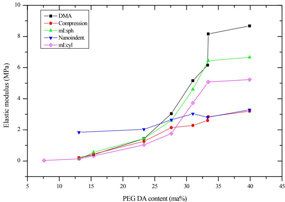
It can be seen that the correlation between the different methods is best for materials with medium stiffness and elastic moduli around 1 MPa. Both for very soft as well as very stiff materials the relative deviations between the different methods are getting larger.
