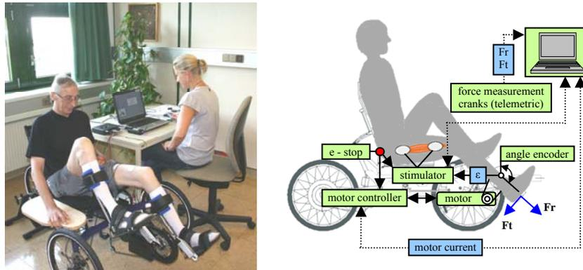
**Figure 1:** The cycling and measurement system during measurements and schematic of control
