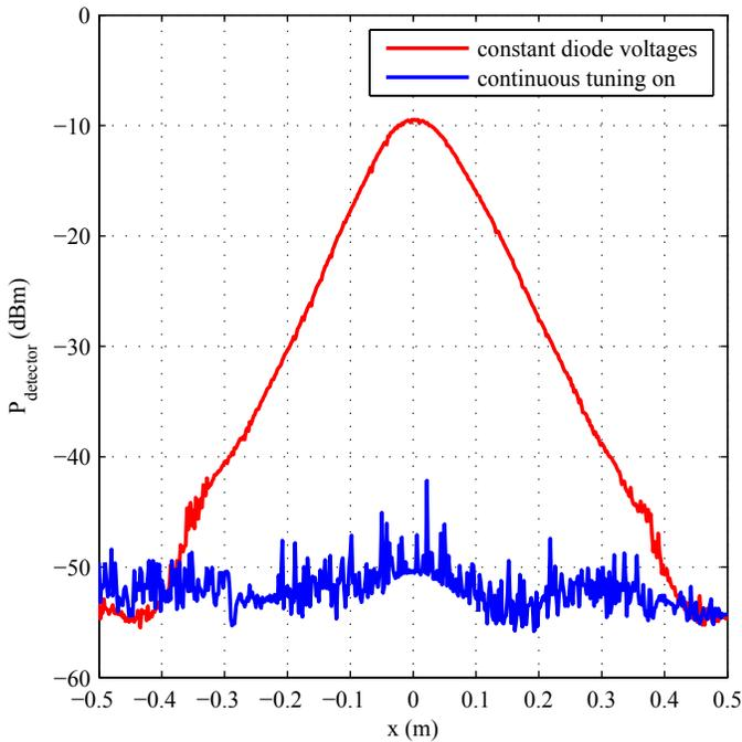
Fig. 3. Detector power (equivalent to receive port power) versus position of a metal reflector sweeping past the antenna on a conveyor belt. At  $x = 0$  m the metal resides directly in front of the antenna.
