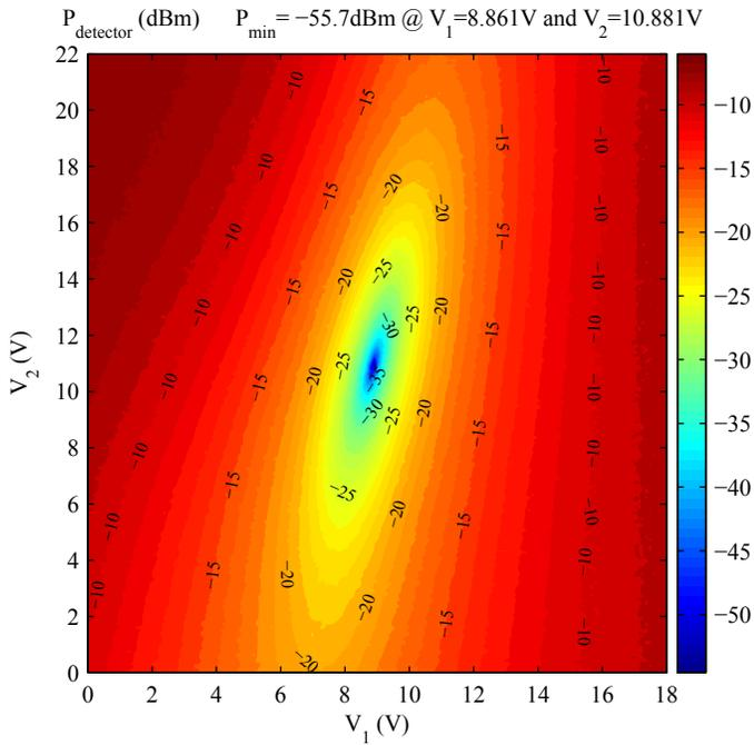
Fig. 2. Output power versus diode tuning voltages  $V_1$  and  $V_2$ .
