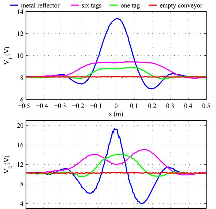
Fig. 4. Automatically tuned varactor voltages  $V_1$  and  $V_2$  during test runs with a metal reflector, one single RFID transponder, and 6 transponders positioned next to each other on the conveyor belt passing by the antenna. For reference, a measurement with the empty conveyor belt is also shown.
