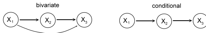
Figure 3.7: Difference of using the bivariate and the conditional Granger index: Contrary to the conditional analysis, the pair-wise case indicates an additional arrow, showing the problem of indirect influence.
