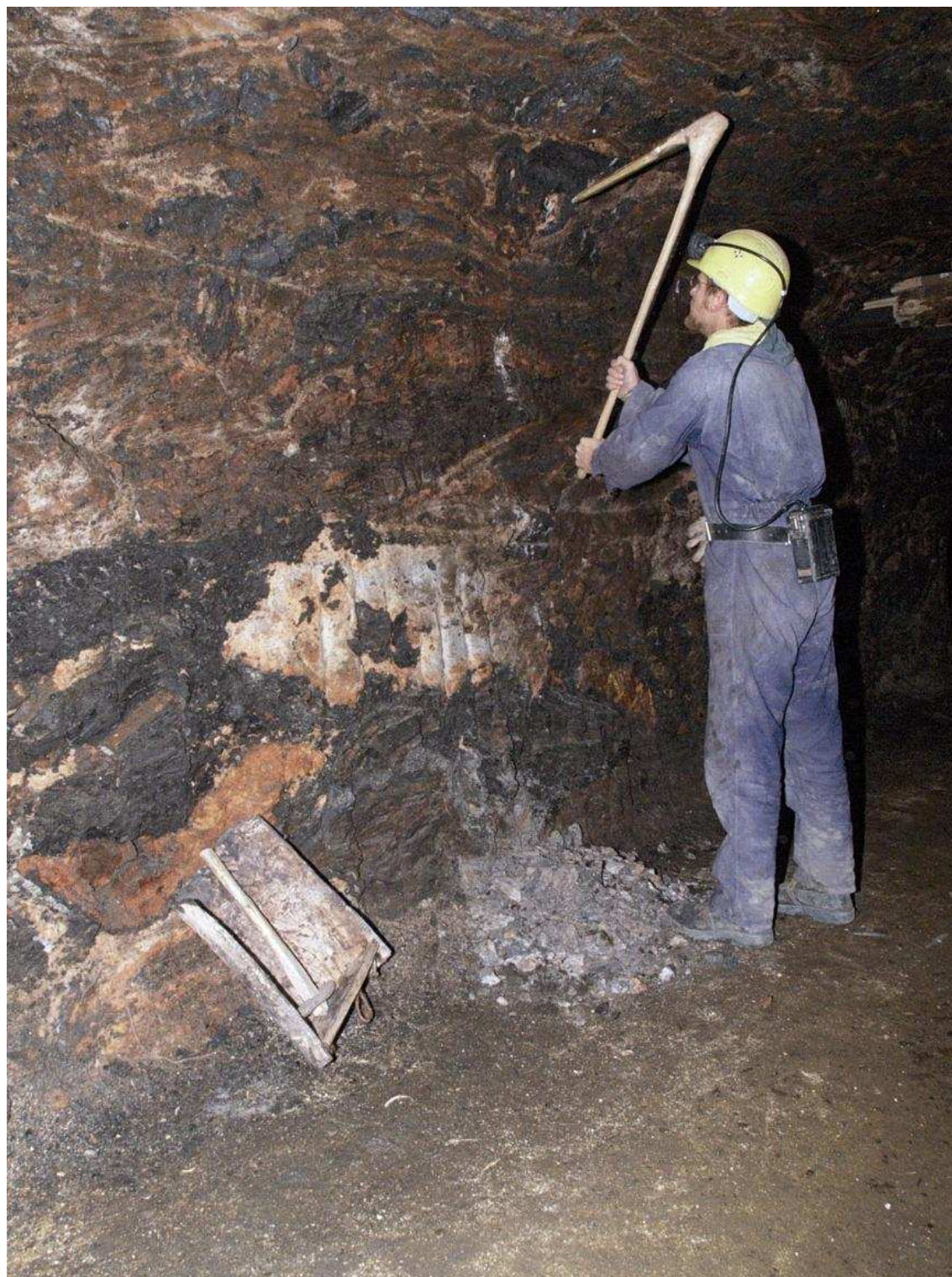
Fig. 10 - Breaking salt with a bronze pick as it was used in the Bronze Age salt mines (©A. Rausch, NHM Wien).
