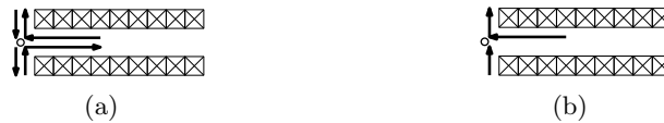
Figure 3.5.: Figure (a) shows a module representing that part of a tour entering and leaving the RA from and to the left side. This aisle operation is then suitably joined with the rest of the tour by appropriate inter-aisle operations.
