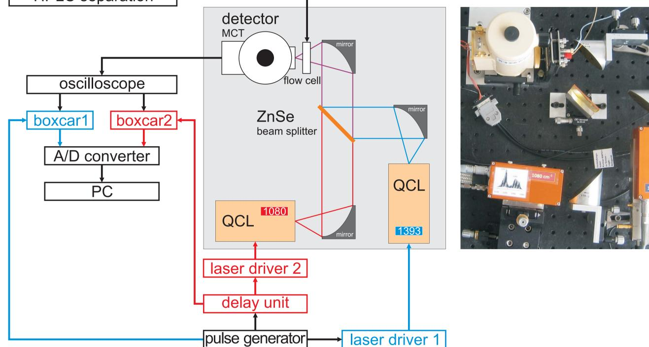
The detector signal is separated electronically using boxcar averagers, processed via A/D converter and stored on a PC.
