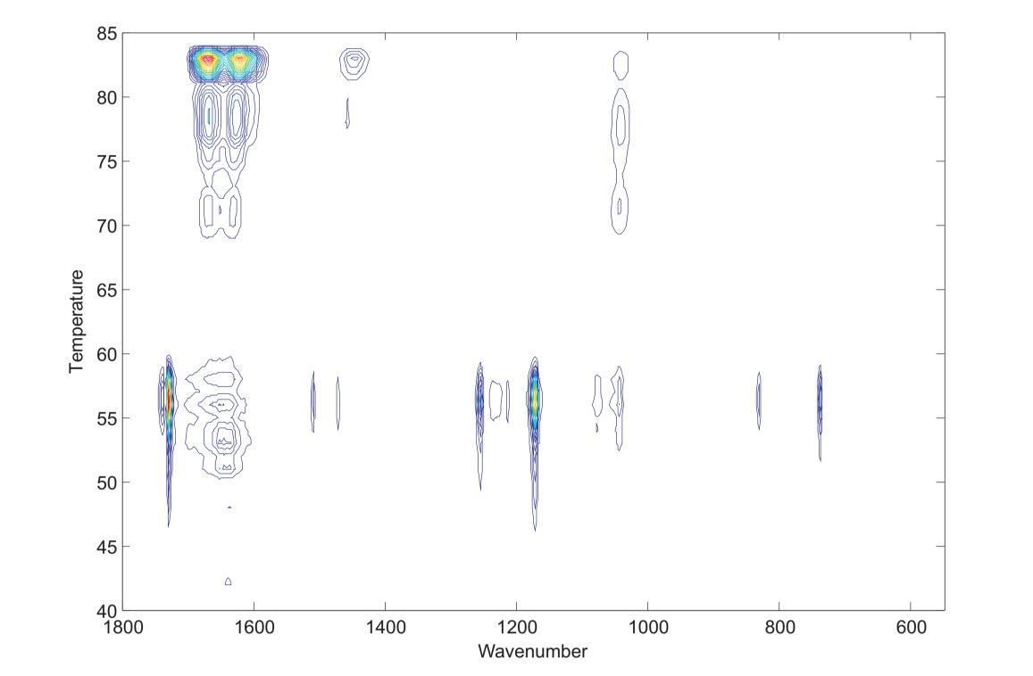
The figure above shows the IR spectra obtained for each temperature for the highlighter pen ink. The pictures on the right show the visible image of the ink obtained at 45, 53 and 65 °C.
