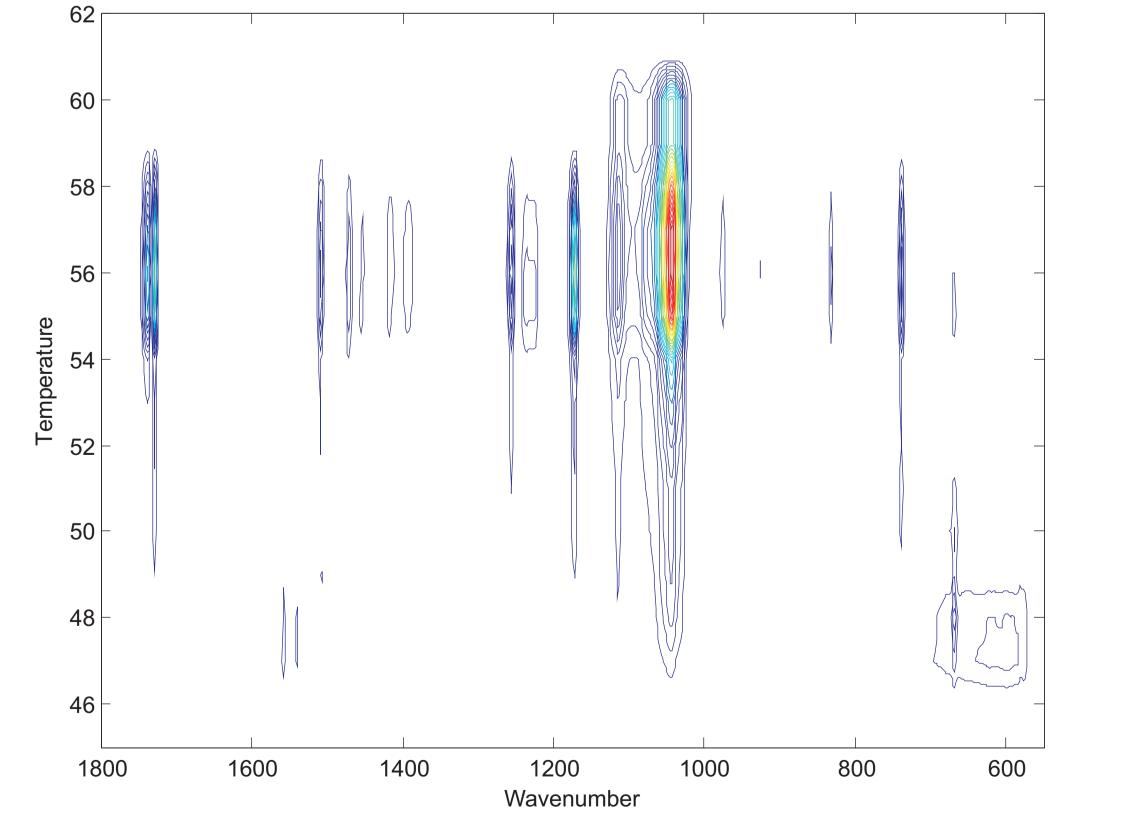
The figure above shows the 2D Correlation moving window plot of the temperature induced IR spectra shown at the top of this panel. (Moving window size was 5 spectra).
