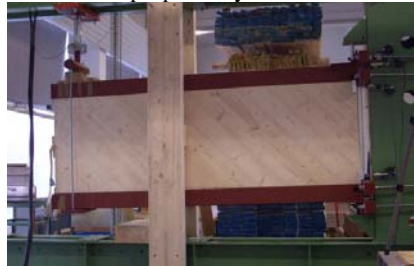
Fig 4. Dynamic testing of hybrid wall system with inclined boards
