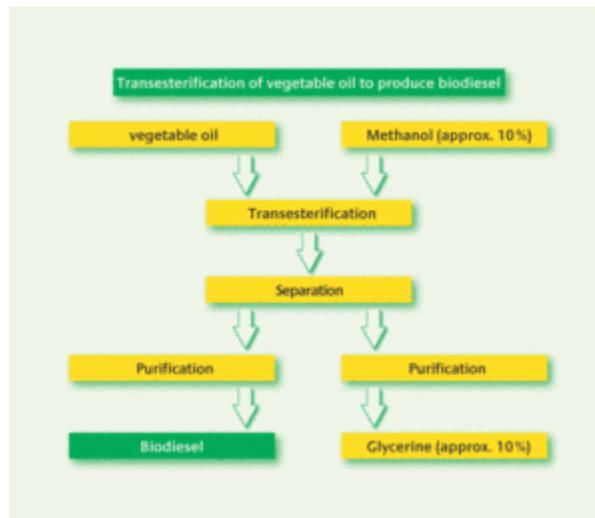
Fig. 15 - Basic transesterification process for converting oils and fats into biodiesel.
