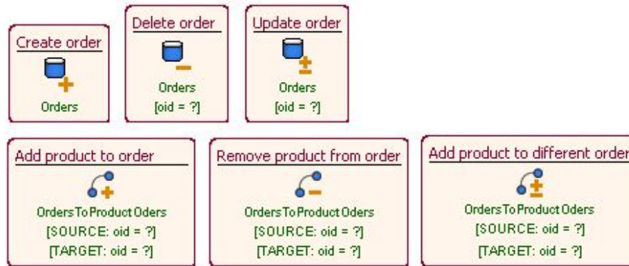
Figure 5.4: WebML operation units. From left to right: CreateUnit, DeleteUnit, ModifyUnit, ConnectUnit, DisconnectUnit, ReconnectUnit.
