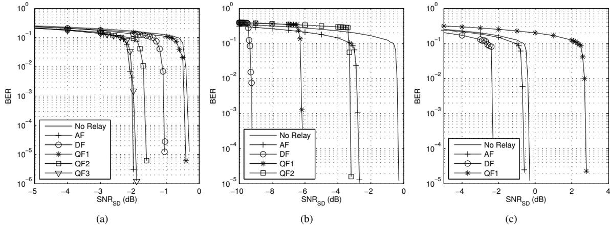
**Fig. 3.** Bit error rate versus source-destination SNR in fast fading: (a) relay near destination ( $d = 0.9$ ), (b) relay halfway between source and destination ( $d = 0.5$ ), (c) relay near source ( $d = 0.1$ ).
