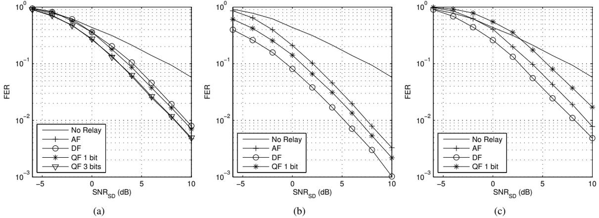
**Fig. 2.** Frame error rate versus source-destination SNR in block fading: (a) relay near destination ( $d = 0.9$ ), (b) relay halfway between source and destination ( $d = 0.5$ ), (c) relay near source ( $d = 0.1$ ).
