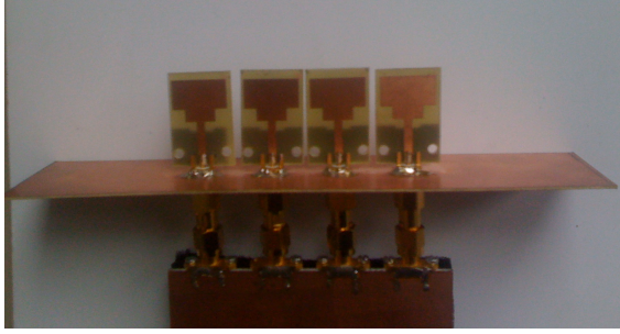
Fig. 5. Four UWB monopole antennas arranged linear with introduced groundplane.
