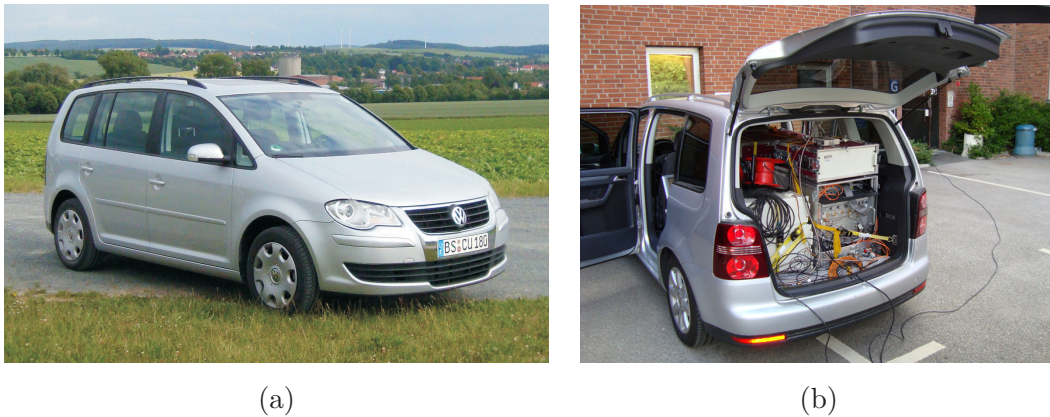
Figure 4.12: (a) Measurement vehicle and (b) Rx vehicle equipped with the channel sounder
