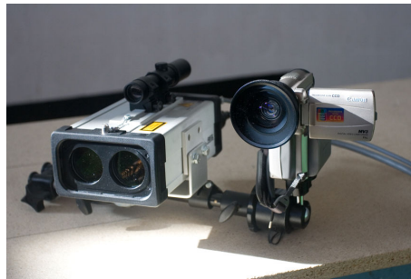
Figure 4.5: Laser distance meter and video camera for documentation
