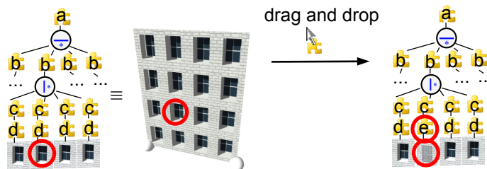
Figure 3.3: On the left, the automatically generated shape hierarchy corresponding to the facade in Figure 3.2 is shown. Only the second floor is visualized, in order to increase readability. Utilizing direct control, the user can drag and drop the desired window on the rendered facade, automatically changing the underlying shape hierarchy, as seen on the right. No manual rewriting is necessary for the user.
