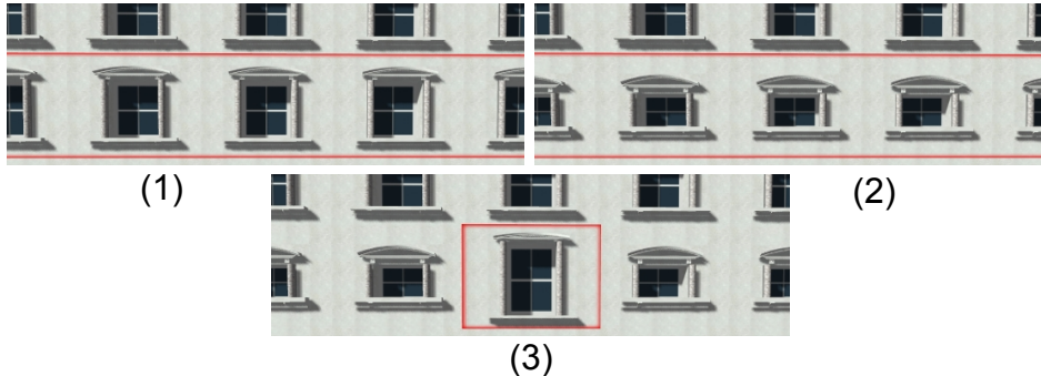
Figure 3.13: Sequence showing hierarchical modifications. (1) A shape representing a floor is selected. (2) The parameter windowHeight is modified - all shapes on lower levels are automatically modified (3) Selecting a specific shape allows overriding the parameter on a lower level.
