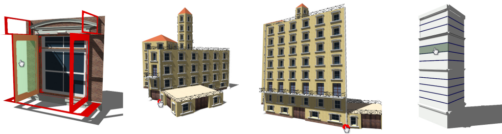
Figure 3.1: Screenshots from our real-time editor for grammar-based procedural architecture. Left: Visual editing of grammar rules. Middle left: Direct dragging of the red ground-plan vertex and modifying the height with a slider creates the building on the middle right. While dragging, the building is updated instantly. Right: Editing is possible at multiple levels, here the high-level shell of a building is modified.
