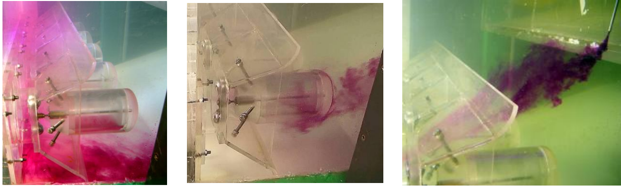
Figure 3-6. Variant 1, bottom near flow, flow around generator bulb and flow field after skimming wall
