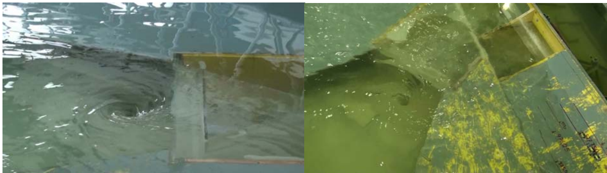
Figure 4 air entraining vortex at 3-out (left case 5, right case 6b)
