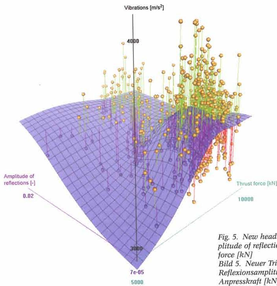
Fig. 5. New headrace tunnel at Hieflau, relationship of amplitude of reflections [-], TBM vibration [ $\text{m/s}^2$ ] and thrust force [kN]
