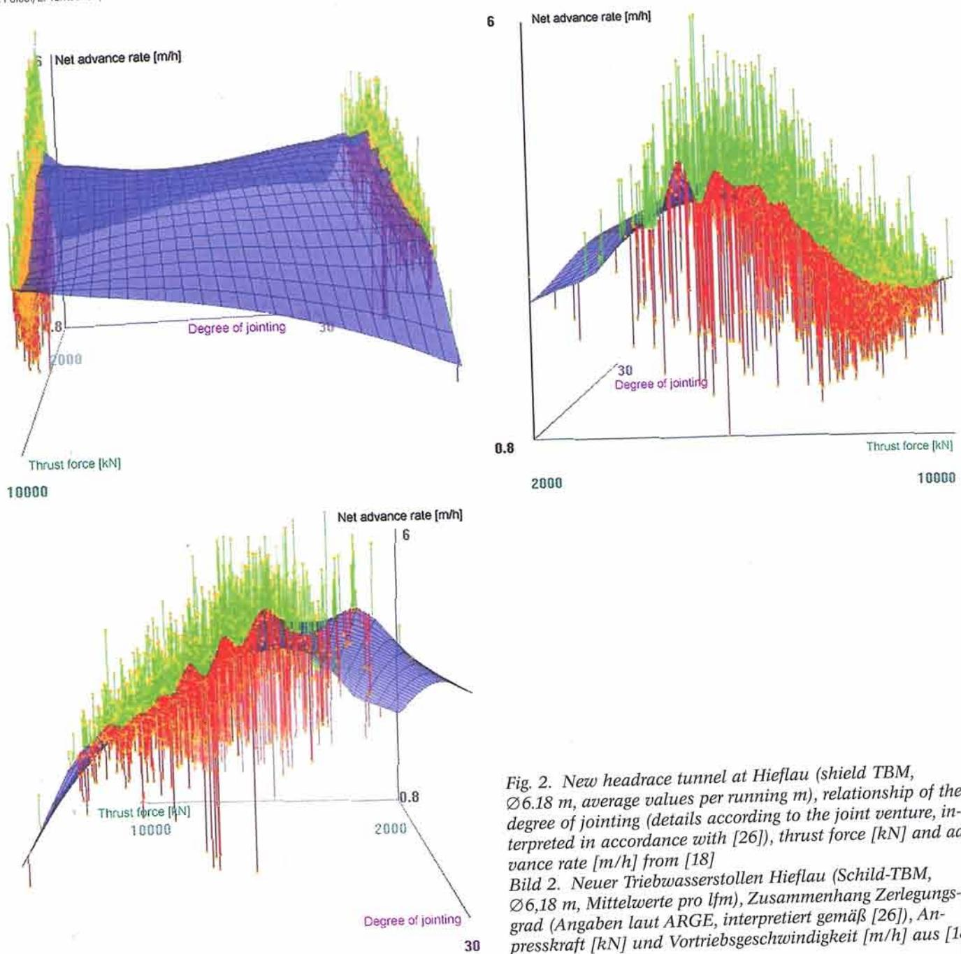
Fig. 2. New headrace tunnel at Hieflau (shield TBM, Ø 6.18 m, average values per running m), relationship of the degree of jointing (details according to the joint venture, interpreted in accordance with [26]), thrust force [kN] and advance rate [m/h] from [18]
