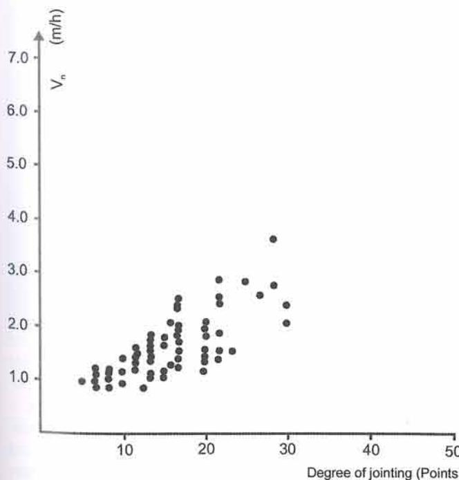
Fig. 1. Relationship of the advance rate to the degree of jointing of the rock mass in the pressure tunnel of the lower stage of Sellrain-Silz power station group (open TBM, Ø3.9 m, daily average values); left: granite gneiss, right: paragneiss and mica schist
