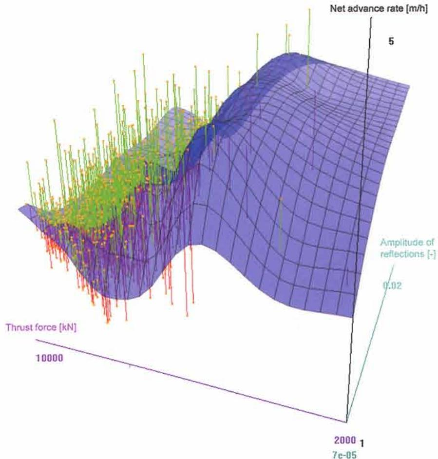
Fig. 3. New headrace tunnel at Hieflau, relationship of amplitude of reflections [-], thrust force [kN] and net advance rate [m/h]
