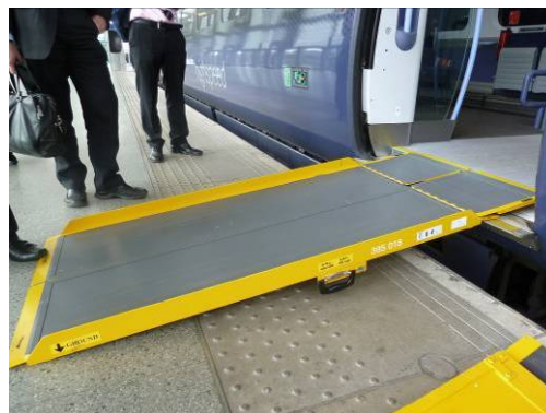
Pic. 20: Manual mobile Ramp (Port-a-Ramp, UK) to bridge the gap between the train and the platform (South Eastern Trains, England)
