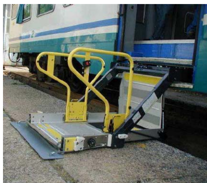
Pic. 57: Cassette Lift (RICON Mirage, used at FS – Italien)
