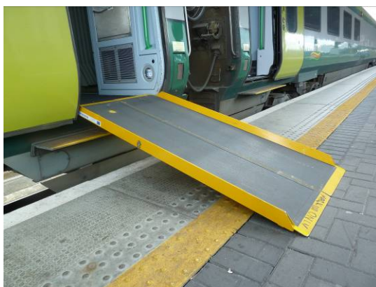
Pic. 18: Ramp as used by Irish Railways (Port-a-Ramp, UK)
