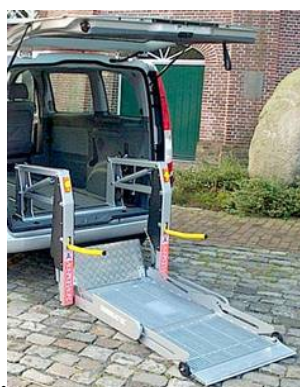
Pic. 99: Linear Lift, horizontal/vertical split-platform (left: AMF-Bruns, right: BraunCorp, )
