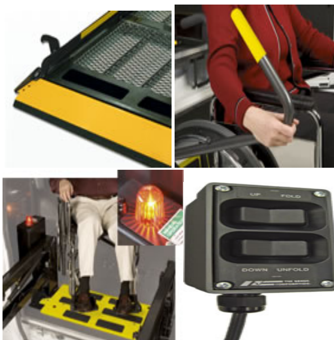
Pic. 100: Automatic Mechanical Roll-stop (far left), Safety Handrails for wheelchair occupant and companion (left), thresh-hold plate locating wheelchair (right), hand-held remote-control for companion (far right)
