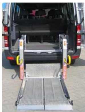
Pic. 99: Linear Lift, horizontal/vertical split-platform (left: AMF-Bruns, right: BraunCorp, )
