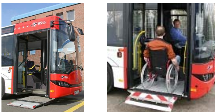
Pic. 92: Floor-Integrated Lift, lifting-column version (MBB Palfinger MEDILIFT LB 300)
