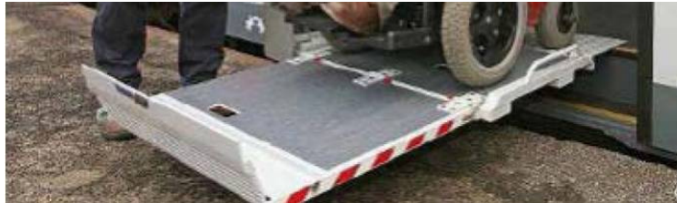
Figure 2.44: Pivoting lift roll-off barrier (MBB Palfinger Trainlift TR 1)
