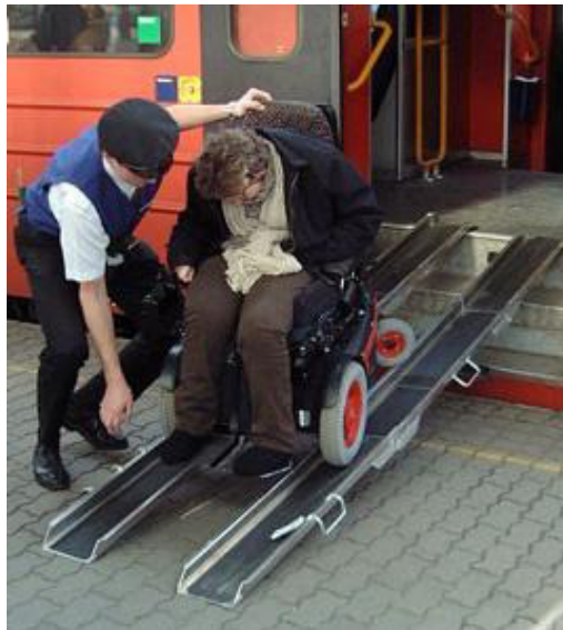
Figure 2.30 Ramp consisting of two separate tracks
