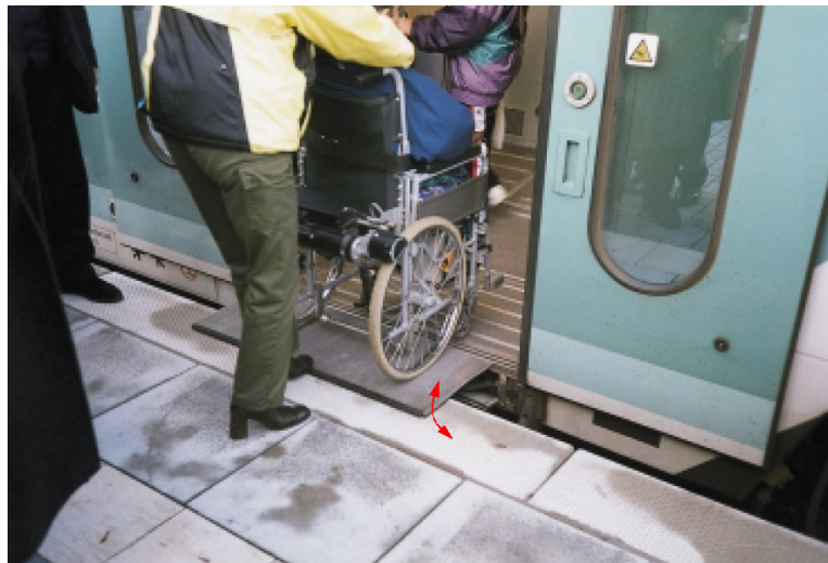
Figure 2.21: Bridging plate with rotational mechanism
