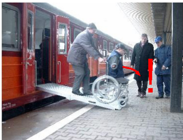
Figure 2.25: Potential risk for wheelchair user to fall down on steep ramps
