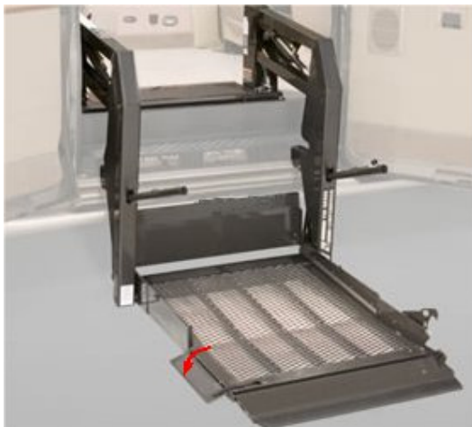
Figure 2.55: Collapsible side barrier- BraunAbility Millennium Series lift
