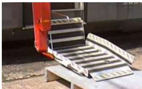
Figure 2.43: Linear lift (U-Lift) side barriers
