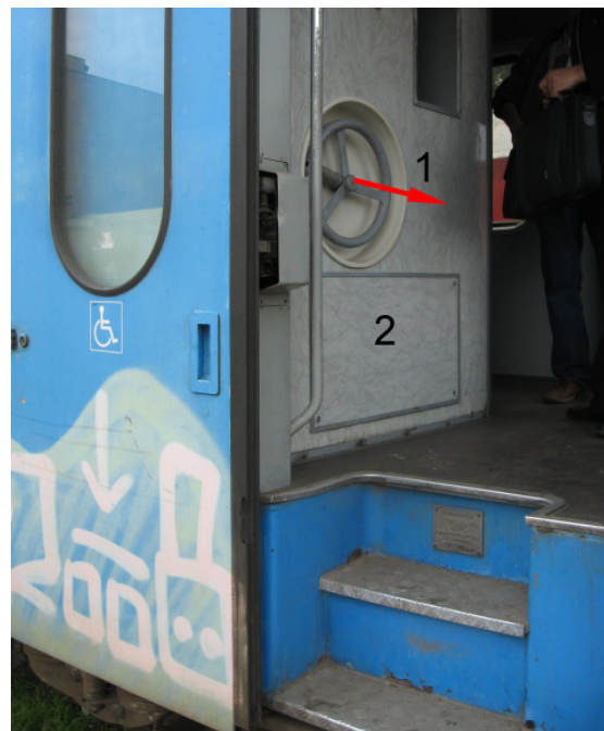
Figure 3.21: Necessary hand brake wheel shift
