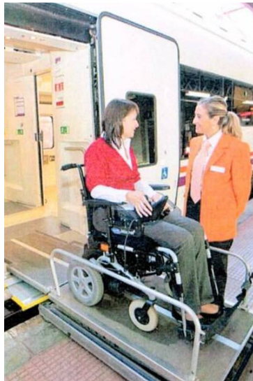
Figure 2.15: Operation of a wheelchair lift by Atendo personnel
