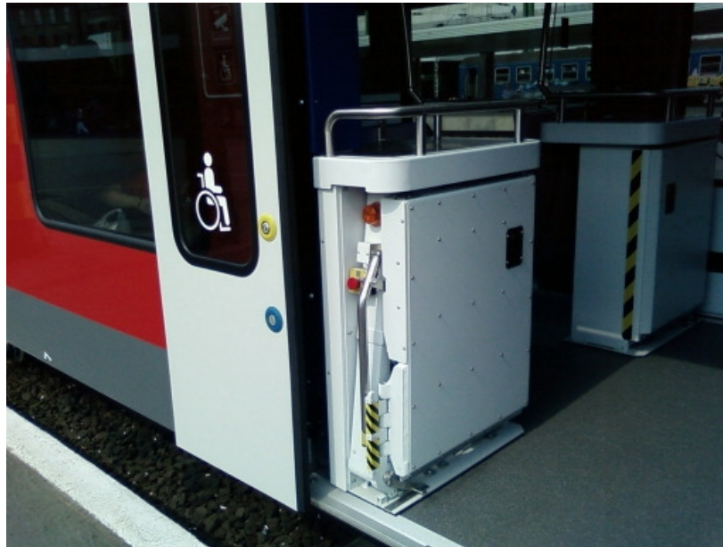
Figure 2.48: Stowed lift at Stadler train (MAV Hungarian Railway)
