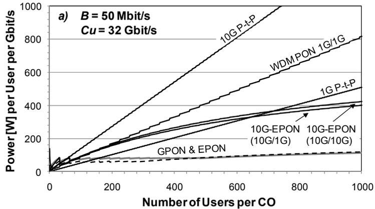
Figure 2. Results on power efficiency for  $C_u = 32$  Gbit/s and  $B = 50$  Mbit/s
