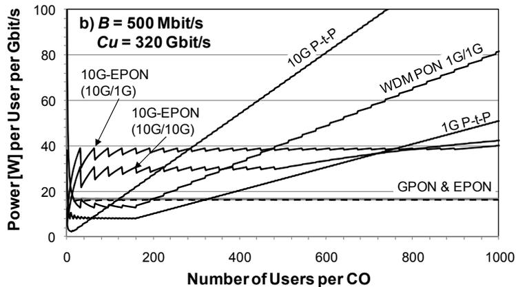
Figure 2. Results on power efficiency for  $C_u = 320$  Gbit/s and  $B = 500$  Mbit/s
