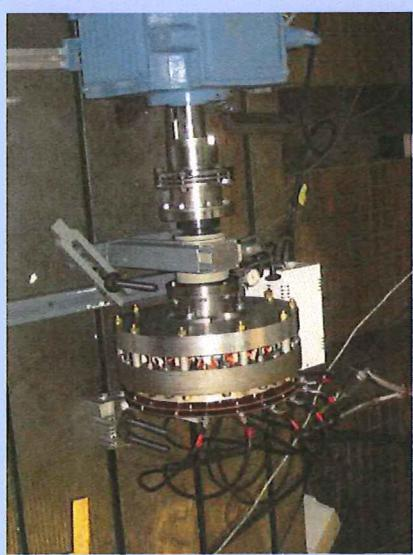
Outer rotor motor with tooth coils
