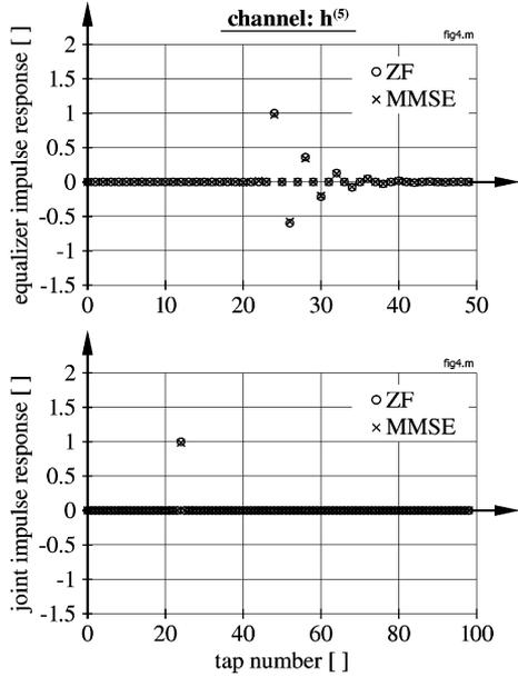
Fig. 5. Upper: ZF and MMSE equalizer impulse response for  $h^{(5)}$ . Lower: Corresponding convolution of channel and equalizer for  $h^{(5)}$ .
