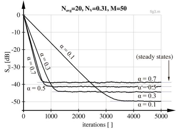
Fig. 3. System mismatch over adaptation steps for various values of  $\alpha$  in noisy NLMS algorithm.
