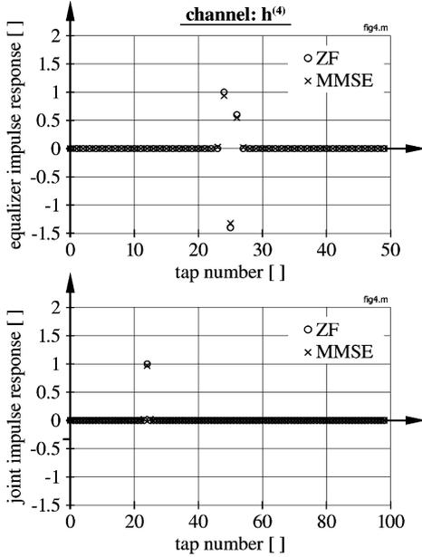
Fig. 4. Upper: ZF and MMSE equalizer impulse response for  $h^{(4)}$ . Lower: Corresponding convolution of channel and equalizer for  $h^{(4)}$ .
