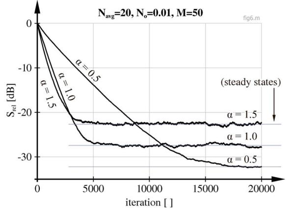
Fig. 6. MMSE equalizer with normalized step-size on channel  $h^{(4)}$ .
