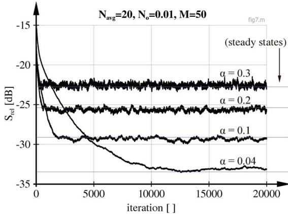
Fig. 7. ZF equalizer with normalized step-size on channel  $h^{(4)}$ .
