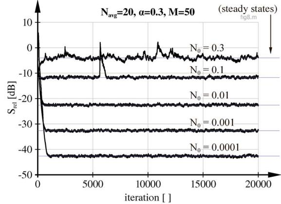
Fig. 8. ZF equalizer with fixed normalized step-size on channel  $h^{(4)}$  when varying additive noise variance  $N_0$ .
