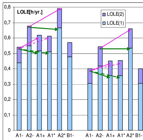
Fig. 2: System-supply-reliability indices for different fault-clearing strategies
