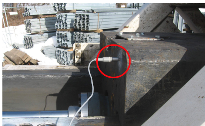
Figure 2. Acceleration sensor mounted on the falling weight of 9,000 kg.
