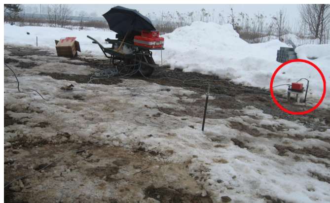
Figure 4. Measurement chain and acceleration sensor mounted in the near-field of the compaction foot (right).
