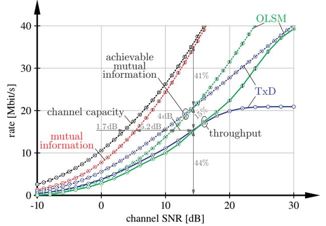
Fig. 10. Throughput of a  $2 \times 2$  system with 5MHz bandwidth compared to the channel capacity, the mutual information, and the achievable mutual information. The small vertical bars within the circular markers indicate the 99% confidence intervals. Reproducible by running *Physical\_Layer\_batch.m*.
