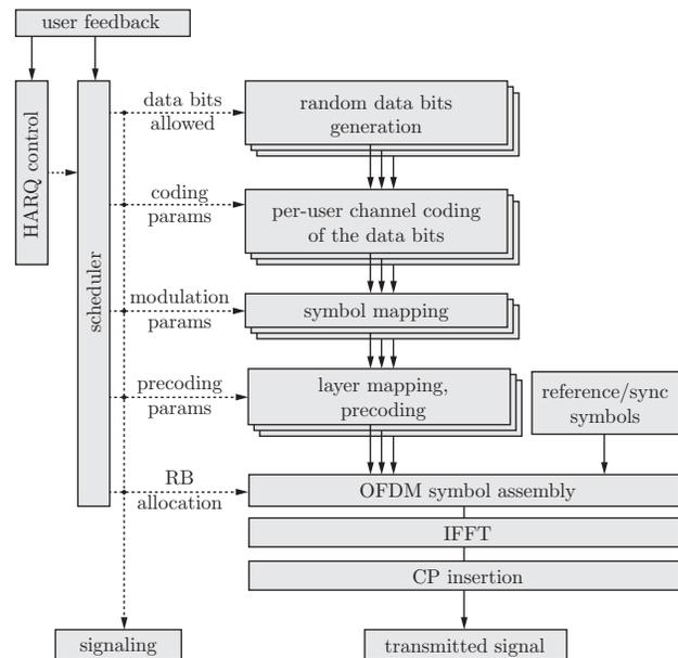
Fig. 2. LTE downlink transmitter structure, as implemented in the Vienna LTE link level simulator.
