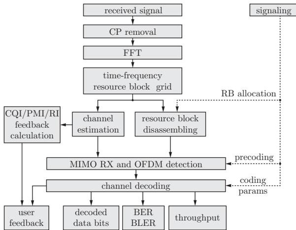
Fig. 3. LTE downlink receiver structure, as implemented in the Vienna LTE link level simulator.
