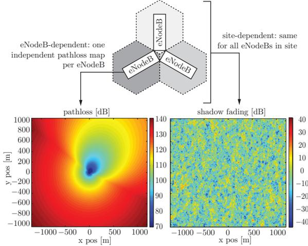
Fig. 7. Left: Large-scale pathloss and antenna gain map [dB] of one eNodeB. Right: space-correlated shadow fading of one site [dB].
