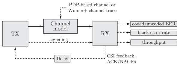
Fig. 1. LTE link level simulator structure, as implemented in the Vienna LTE link level simulator.
