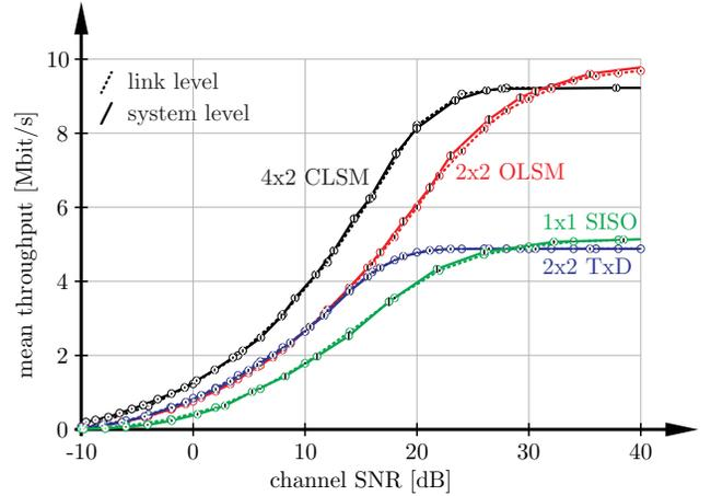
Fig. 9. Cross-comparison of throughput results obtained with the link level and the system level simulators. The small vertical bars within the circular markers indicate the 99% confidence intervals. Reproducible by running *Reproducibility\_LLvsSL\_batch.m*.
