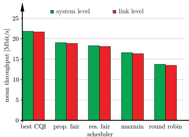
Fig. 11. Comparison of system throughput obtained with different scheduling strategies with link and system level simulations. Reproducible by running *Reproducibility\_Schedulers\_batch.m*.
