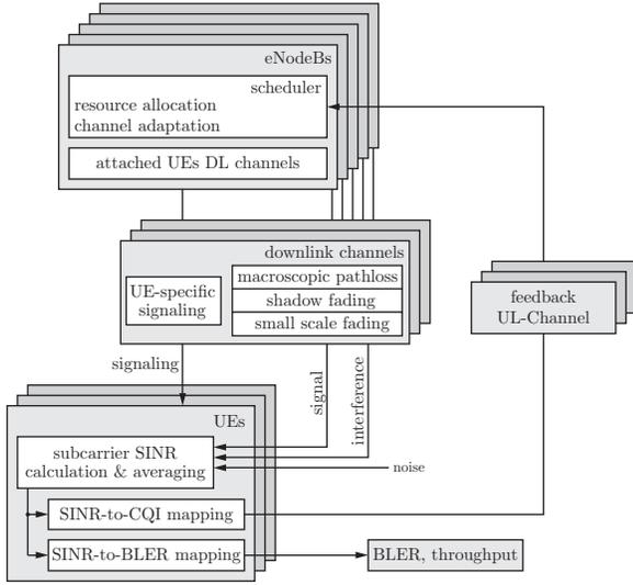
Fig. 6. Schematic class diagram showing the relation between the several components comprising the LTE System Level Simulator.
