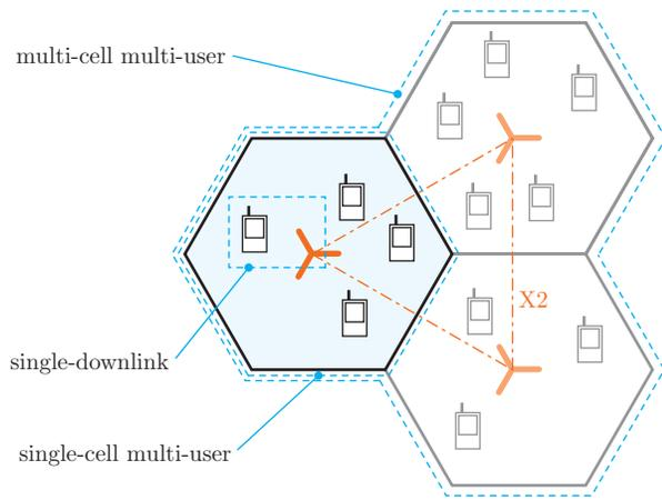
Fig. 4. Three different scenarios in the Vienna LTE link level simulator allow to adjust the scale of the simulation.
