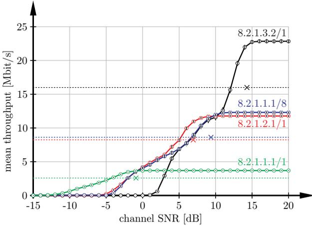
Fig. 8. Throughput simulations of the test scenarios in 3GPP TS 36.101 and comparison to the minimum performance requirements (marked with crosses). The small vertical bars within the circular markers indicate the 99% confidence intervals. Reproducible by running *Reproducibility\_RAN\_sims.m*.
