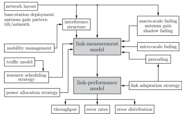
Fig. 5. Schematic block diagram of the LTE system level simulator.
