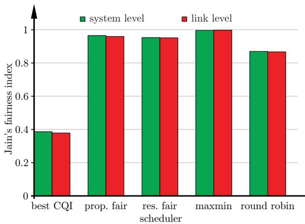
Fig. 12. Comparison of fairness obtained with different scheduling strategies with link and system level simulations. Reproducible by running *Reproducibility\_Schedulers\_batch.m*.
