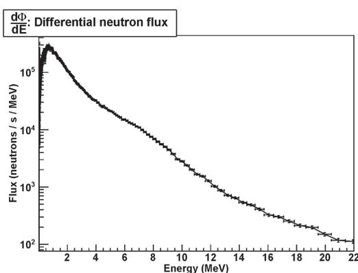
The flux is measured using a <sup>235</sup>U fission chamber. The vacuum evaporated <sup>235</sup>UF<sub>4</sub> deposit is highly enriched in <sup>235</sup>U (>99.5%) and very thin (324  $\mu\text{g}/\text{cm}^2$  of <sup>235</sup>U). The effective thickness of the fission chamber was chosen between 6 and 7 mm, as this leads to the best ratio of fission fragment energy loss (signal) and radioactivity  $\alpha$  particle energy loss (background noise).
