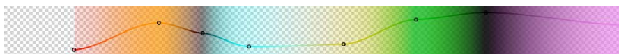
Figure 6.2: Example for a transfer function (TF). The x axis represents the signal range [0, 1] , the y axis the opacity \alpha \in [0, 1] .
