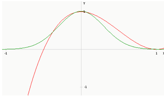
Figure 4.9: The green line describes the Gaussian function in equation 4.5 with a kernel size 1. The red line depicts the cubic attenuation function in equation 4.8. Only the parts of the attenuation functions that are equal to or lie between 0 and 1 on the x-axis are used for attenuation, so strange behaviour due to negative values is excluded.
