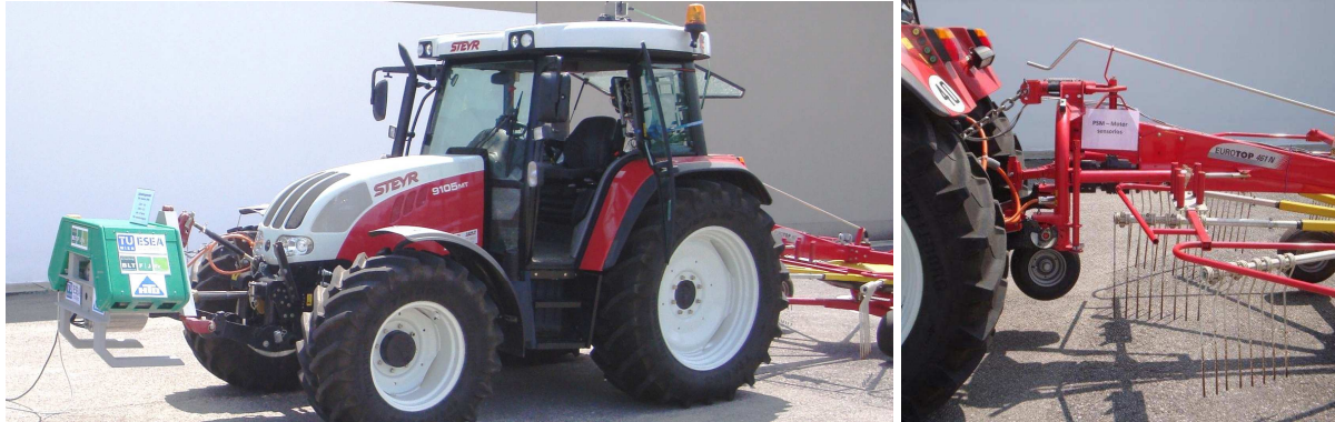
Figure 2: tractor with electric swather powered by the multi-purpose pto generator
