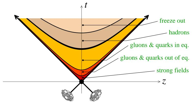
[Gelis 2010] Illustration of the stages of a heavy ion collision.
