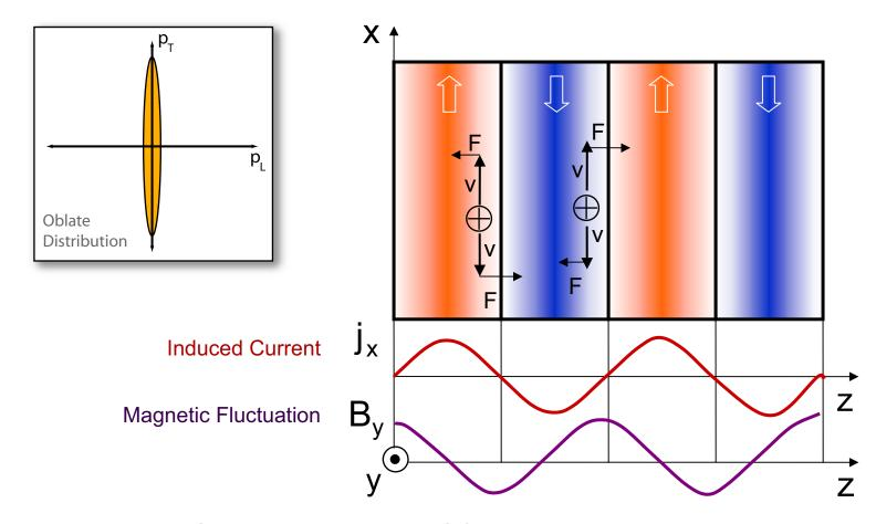
Illustration of the mechanism of filamentation instabilities.
