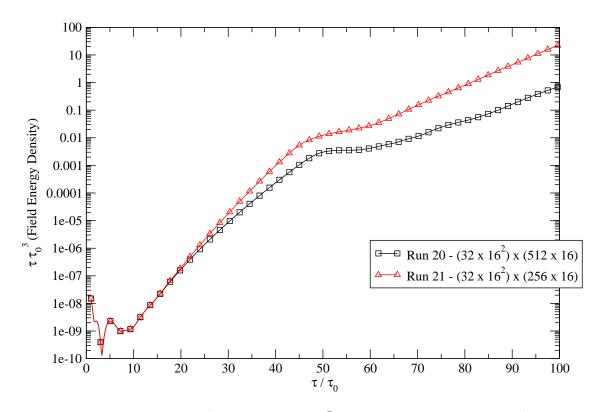
[Attems, Rebhan, Strickland forthcoming] Preliminary runs from the HEL 3d parallell code of a non-Abelian single mode setup with identical longitudinal and transverse lattice sizing, but different W auxiliary field numbers.
