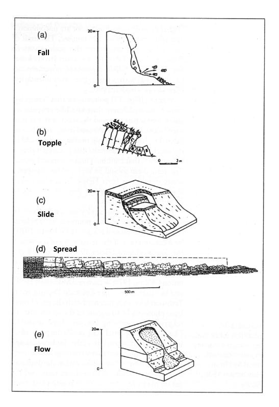
Figure 2: Types of landslides according to Cruden & Varnes, 1996
