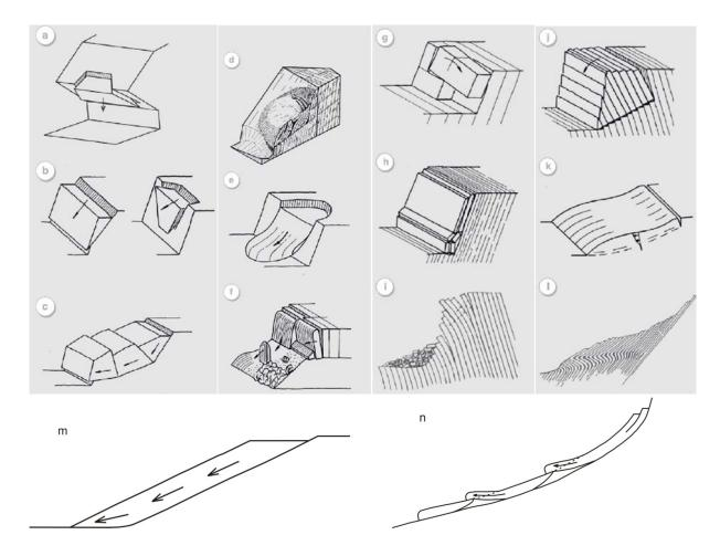
Figure 3: Slope failure mechanisms
