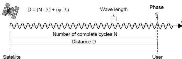
Fig.1 Principle of the phase measurement [2]
