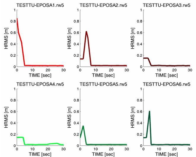
Fig.5 Initiazation of Ashtec ProMark 500 within EPOSA network
