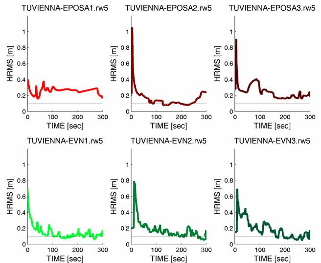
Fig. 8 Initialization of Mobile Mapper 100, within EPOSA and EVN networks – 5min Test
