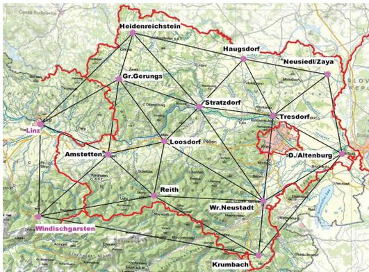
Fig.2 Topography of EVN RTK network among Lower Austria
