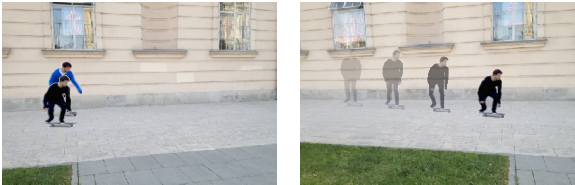
Figure 9.2: Examples of layers and an example for realized post effects as used in the Skateboard Tutor Application; captured from an iPhone 4S. (Left) Playing back two video augmentation layers allows the comparison of the riders' performance. (Right) Flash-trail effects visualize the path and the motion within the video.
