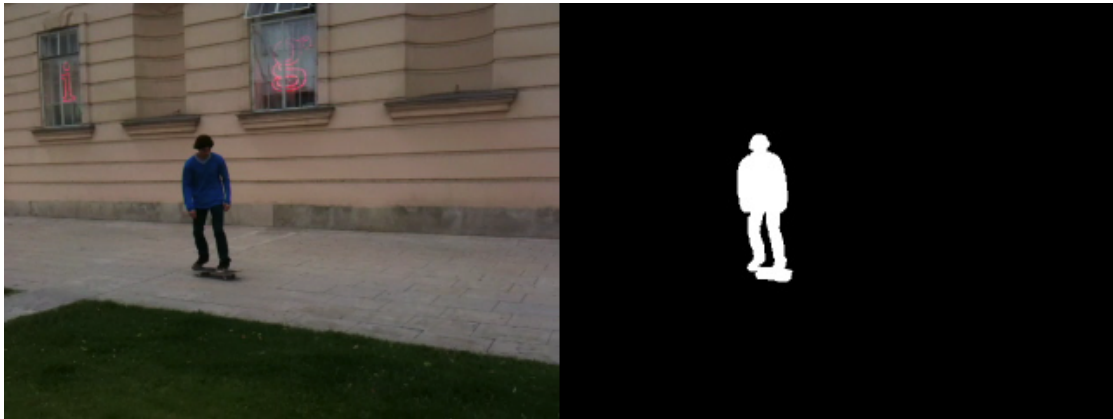
Figure 5.8: Video frame (left) and final alpha mask (right). The white contour resembles the extracted foreground object.
