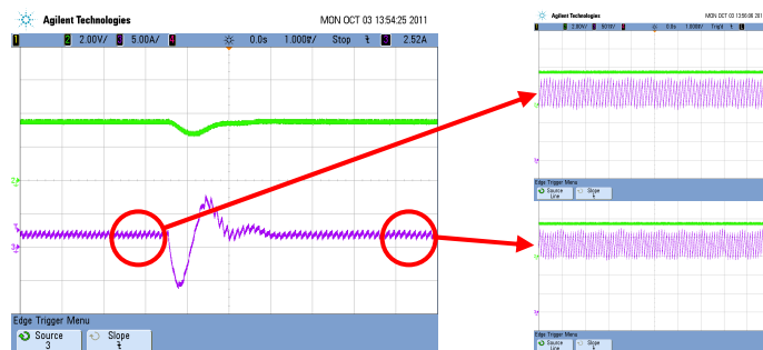
Fig.8: PWM signals of reconfigurable digital interleaved PWM modulator. “Seamless” transition from N=8 to N=7 converter cells (left) and vice versa (right). Also shown: Cell’s PWM on/off control concept (FPGA realization).
