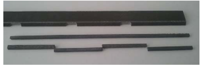
Fig 4: Industrial standard magnetic slot wedge material and adapted slot wedges.
