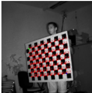
Figure 3.11: A sample of the corner selection with an amplitude image made with the PMD depth camera.
