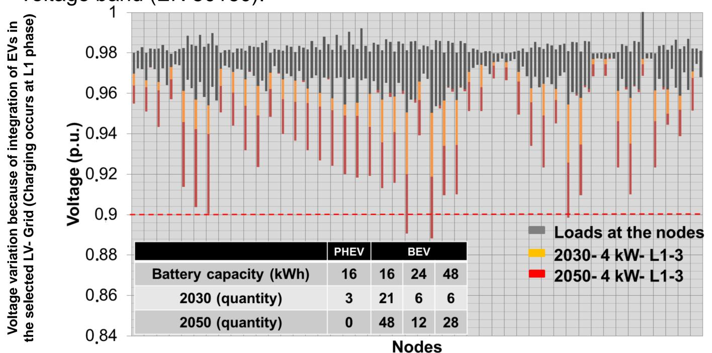
On the other hand, the even distribution of BEVs between all phases has been recommended in this case. In addition enough voltage band will be available for integration of other loads into the LV-Grids.
