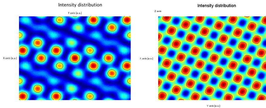
Fig. 4: Intensity distribution of 4 interfering laser beams. Left: Asymmetrical arrangement of the beams around z-axis. Right: Asymmetrical arrangement with different polarisation of 2 beams.
