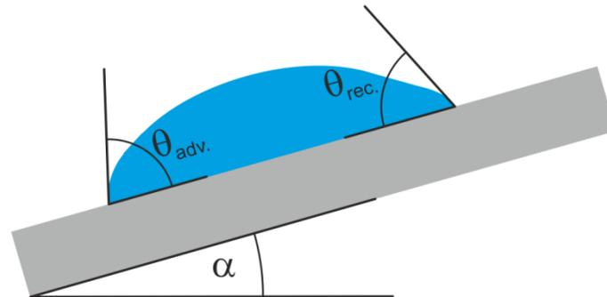
Fig. 1: Contact angle  $\Theta$  and tilt angle  $\alpha$ . Hysteresis of the contact angle is defined as difference between advancing or receding contact angles  $\Theta_{adv.} - \Theta_{rec.}$  of a water droplet and is responsible for „sticking“ of liquids on surfaces [3]. Self-cleaning surfaces show small tilt angles [4].
