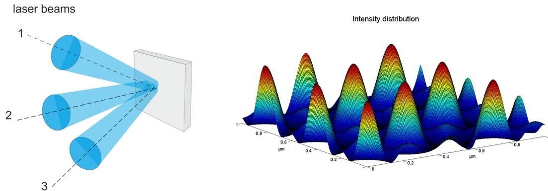
Fig. 2: Schematical view of three interfering laser beams (left). Resulting intensity distribution of interfering beams (right) with identical polarization orientation and amplitude.
