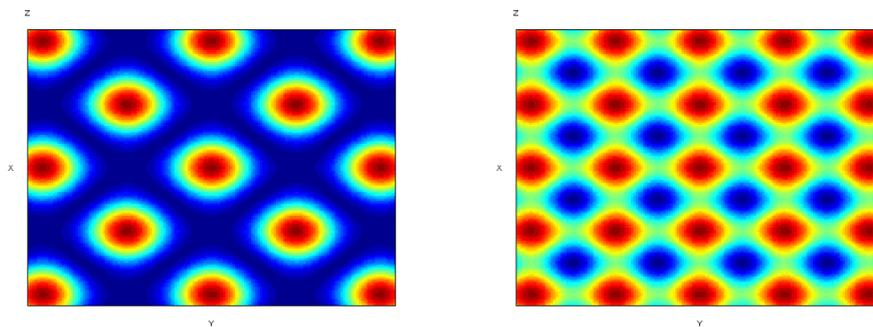
Fig. 3: Calculated intensity distribution of four interfering laser beams at the surface of a sample. Z-axis perpendicular to the paper plane. Beams are symmetrically distributed around the z-axis and at angle of  $35^\circ$  from the z-axis. Orientation of polarization identical for all four beams. Left: No phase shift between individual beams. Right:  $90^\circ$  phase shift between beam 1 and beam 3.
