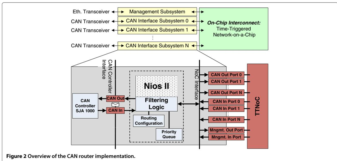
Figure 2 Overview of the CAN router implementation.
