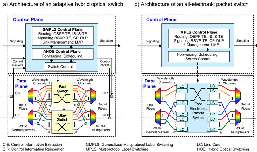
**Figure 3.** Architectures of a) an adaptive hybrid switching node and b) an all-electronic packet switching node.
