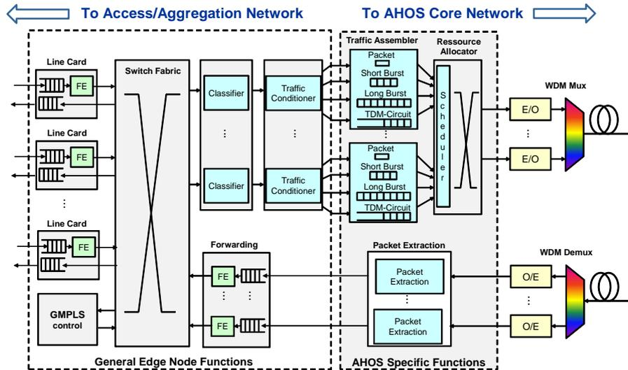
**Figure 4.** Generic architecture of an AHOS edge node (FE: Forwarding Engine, O/E: Optical/Electrical Conversion, GMPLS: Generalized Multiprotocol Label Switching, WDM; Wavelength-Division Multiplexing)
