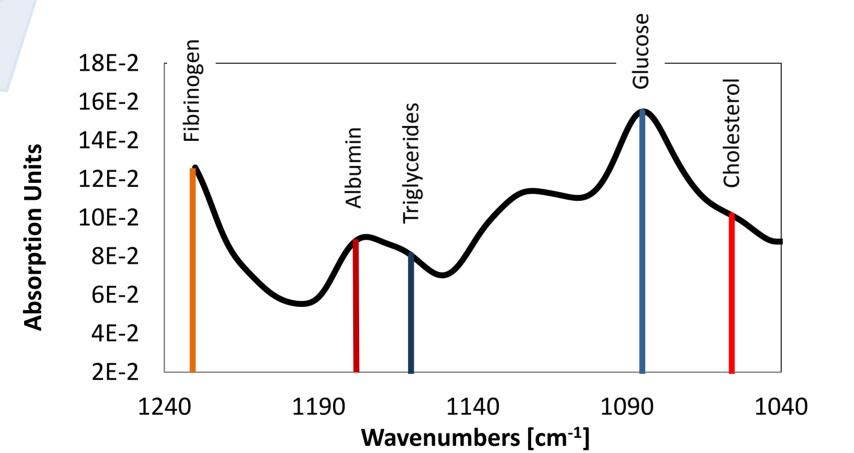
Typical spectrum of human blood plasma; the spectral positions of the absorption maxima of the pure analytes of interest are denoted in the spectrum.
