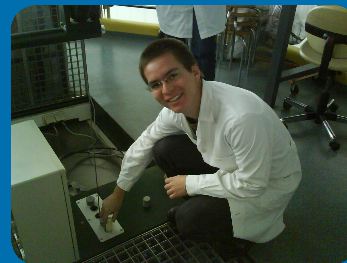
Fig. 4: Inserting irradiation sample holder into the first of the five reflector irradiation tubes of the TRIGA Mark II reactor, filled with a \text{Tb}(\text{NO}_3)_3 sample.
