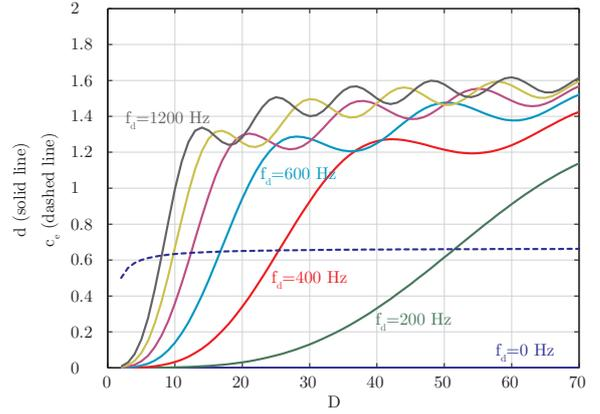
Fig. 2. Coefficients  $c_e(D)$  and  $d(D, f_d)$  over distance between two adjacent pilot-symbols for an LS channel estimator for various maximum Doppler frequencies.
