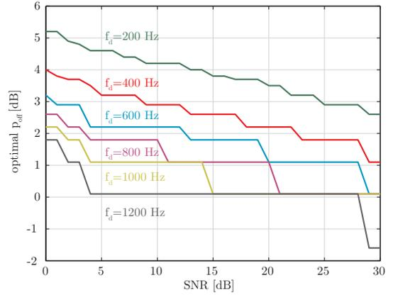
Fig. 4. Optimal choice of the ratio of the pilot power and data power  $\frac{\sigma_p^2}{\sigma_d^2}$  over SNR for values of the maximum Doppler frequency  $f_d$ .
