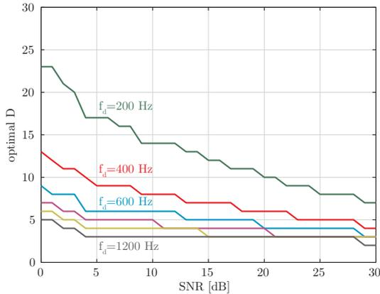
Fig. 3. Optimal choice of the distance between adjacent pilot-symbols  $D$  over SNR for values of the maximum Doppler frequency  $f_d$ .
