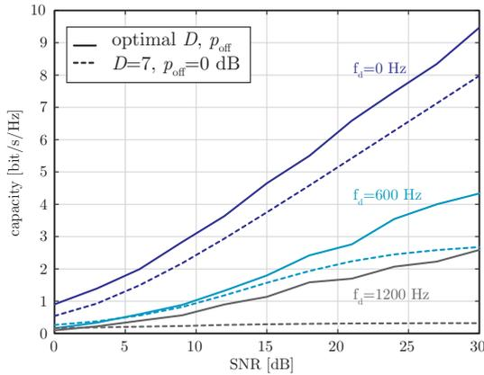
Fig. 5. Capacity versus SNR for system with optimal pilot distance  $D$  between pilot-symbols and optimal power offset  $p_{\text{off}}$  (solid line) and for system with fixed distance between pilot-symbols ( $D = 7$ ) and no power distribution (dashed line).
